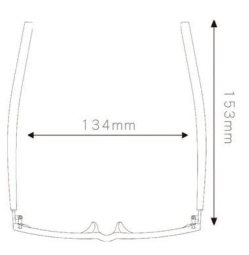
It is normal to have 1-3mm error when the injection dimension is measured by hand
